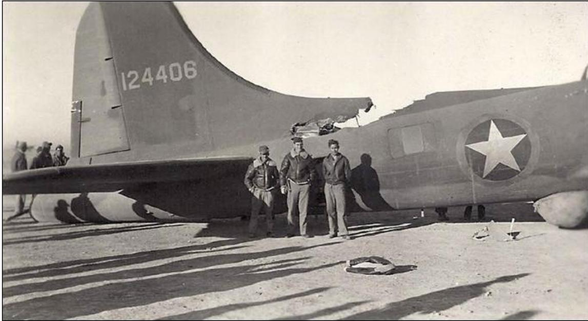
Although the tail actually bounced and swayed in the wind And twisted when the plane turned and all the control cables were severed, except one single elevator cable still worked, and the aircraft miraculously still flew!
