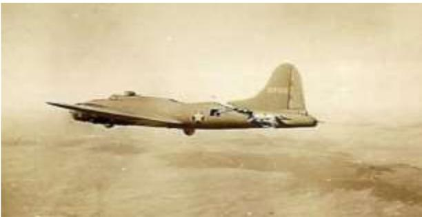
Although the tail actually bounced and swayed in the wind, and twisted when the plane turned. And all the control cables were severed, except one single elevator cable still worked, and the aircraft miraculously still flew!
