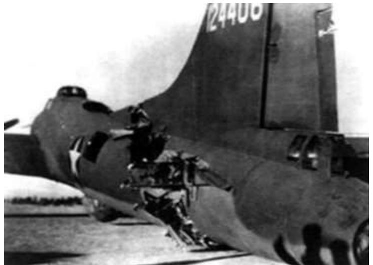
The Fortress sat placidly until the crew all exited through the door in the fuselage and the tail gunner had climbed down a ladder, at which time the entire rear section of the aircraft collapsed.
